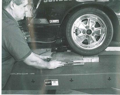
Above: Chapman rolls the car onto the scales from the wooden blocks. Then he jostles the car up and down to settle the car onto its suspension. Empty, Siciliano's 911 weighed 2,100 lbs.
